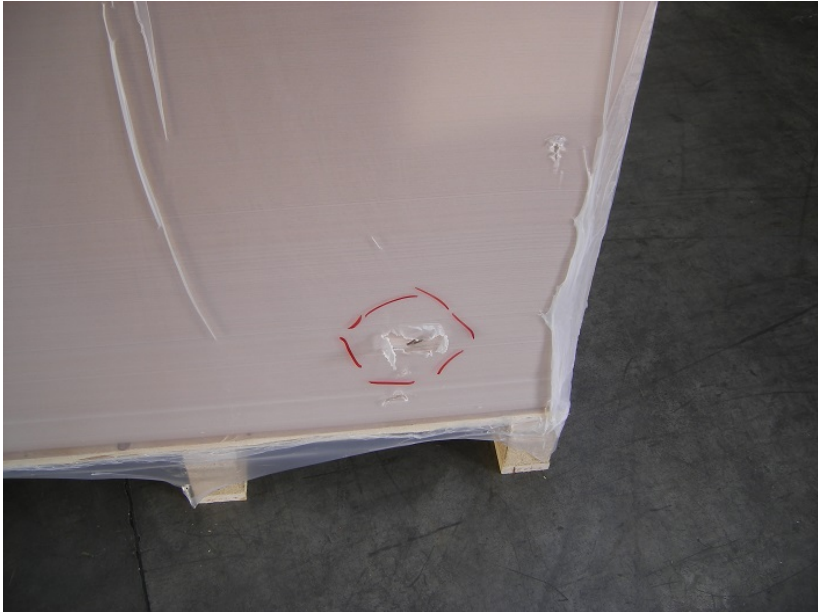
Ok to tape but inform customer about damaged sheets.
